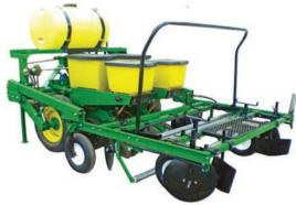
**Plants** 2 rows of sweet corn in furrows. 22" between rows. Between plant spacing 16"-30" and is easily adjustable. Uses John Deere 7000 series row units with precision planting finger meters, seed firmer and rubber closing wheels. The 2 furrow openers are 12" double discs that are adjustable in height with pin.
