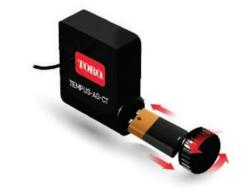
Tempus control units are powered by a 9V battery. The system will alert you when there is 20% battery life left. Only the base stations require 110 volt or a solar panel to create the network. No grid power is required to operate the system. When using irrigation control valves they have to operate with a 12 volt DC latching solenoid.
