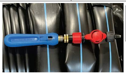
The starter with valve or starter goes on to the insert tool, colored nut to the blue handle. You then use the insert tool to poke a hole and push the fitting into the header hose.
