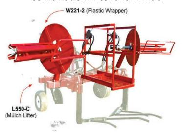
Plastic lifter and winder in one machine, lift and remove 1 row of plastic and drip tape in one pass. Needs two sets of hydraulic remotes, one for the lifter reset and one set of remotes for the winders. Winders have collapsible core for easy removal of tape and plastic.
